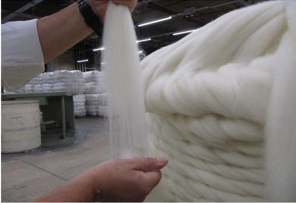
Figure 2: Wool Top- with fibres that have been cleaned and combed<sup>1</sup>. The local industry believes there is a viable business case for the processing of wool up to the point of top production.
